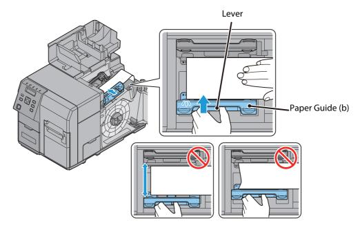
11. Insert the end of the paper into the paper feed slot. The paper starts to feed automatically after a certain amount is inserted.
