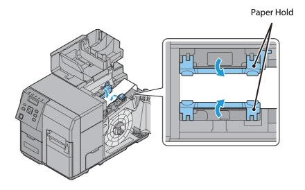
13. If the paper is loose, turn the roll paper flange in the direction of the arrow to tighten the paper.
