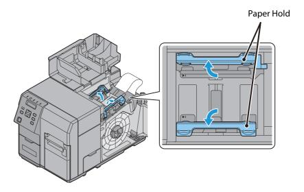
9. Insert the paper along the paper guide (a). Align the end of the paper with ▶ | mark.
