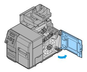
4. Pull out the roll paper flange while holding the release lever of the roll paper flange between your fingers.
